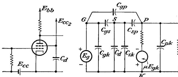
FIG. 4-6. Schematic and equivalent circuits of a tetrode in an amplifier circuit.
