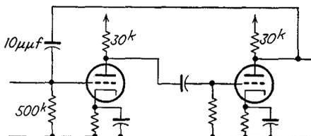
5-16. Calculate the effective input impedance of the circuit in the accompanying diagram.
