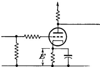
FIG. 7-8. A self-biased grid-circuit limiter.
