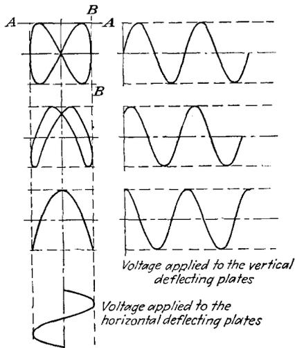
FIG. 22-20. Lissajous figure for 1:2 frequency ratio.
