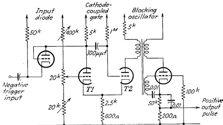
FIG. 19-23. A linear delay multivibrator which triggers a blocking oscillator to produce a sharp pulse.
