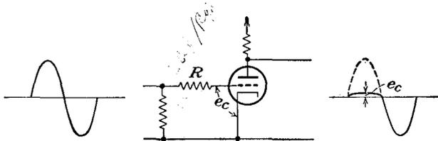
FIG. 7-6. Grid-circuit limiter.
