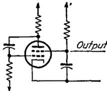
**18-8.** A balanced multivibrator is operated at 1,000 cps. The constants are those of Prob. 18-1 except for the values of  $C_1$  and  $C_2$ . It is to be synchronized by injecting a positive pulse on the grid. What must be the amplitude of the synchronizing pulse if the frequency is 1,100 cps?
