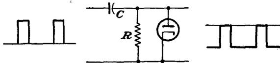
FIG. 7-28. A negative clamping circuit.
