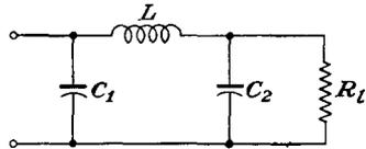
FIG. 14-15. A  $\Pi$ -section filter.
