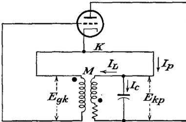
FIG. 12-5. Tuned-plate oscillator.
