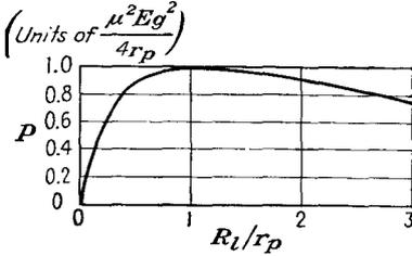
FIG. 9-2. Variation of power output as a function of resistance ratio  $R_l/r_p$ .
