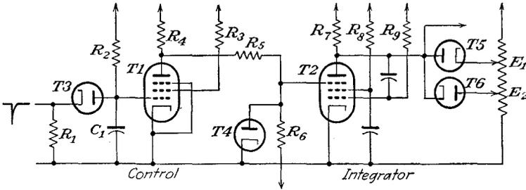
FIG. 19-28. The sanatron delay circuit.
