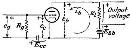
FIG. 3-1. The basic circuit of a triode amplifier.
