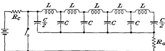
FIG. 19-39. The basic circuit incorporating a pulse-forming line.
