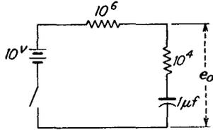
7-4. The interelectrode and wiring capacitances will affect the shape of the output wave form for a given input wave form. Refer to the circuit in the accompanying diagram.
