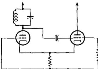
12-4. Using the 806 tube, whose constant current characteristics are given in Chap. 11, calculate the performance when it is used in the oscillator circuit shown in the figure.
