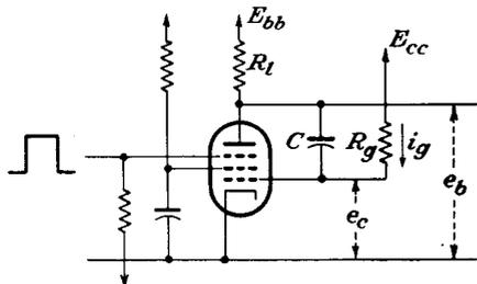
FIG. 19-24. The basic Miller integrating circuit.
