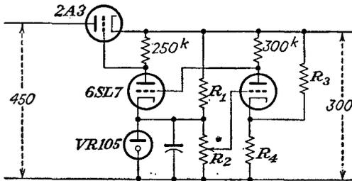
14-13. Design a regulated power supply that will supply 150 ma at 250 volts from a 450-volt rectified and filtered source, with a ripple not to exceed 0.1 per cent and with a stabilization ratio of 15,000. What is the rms ripple voltage in the output of this regulated source if a  $\Pi$  filter consisting of two  $8\text{-}\mu\text{f}$  capacitors and a 12-henry choke is used? The effective output resistance is 650 ohms.
