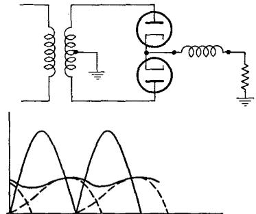
FIG. 14-3. Full-wave rectifier circuit with inductance choke, and the wave shape of the load current.
