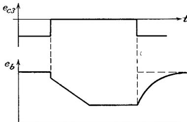
FIG. 19-25. The suppressor and plate potential of the Miller integrating circuit of Fig. 19-24.
