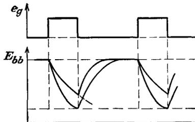
FIG. 20-14. The output-voltage wave form from the sweep generator of Fig. 20-13.
