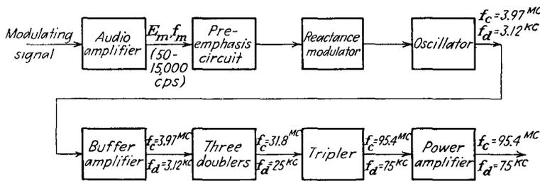
FIG. 17-9. A simple reactance-tube f-m transmitter.
