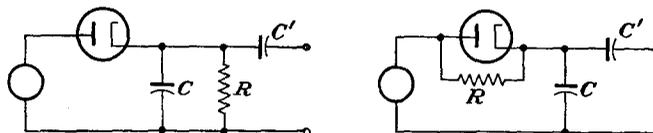
FIG. 16-3. Two circuits for envelope detection.
