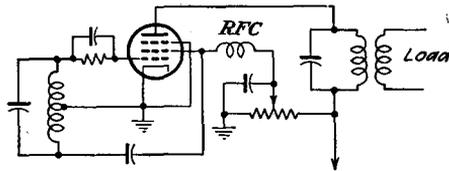
FIG. 12-8. Electron-coupled oscillator.
