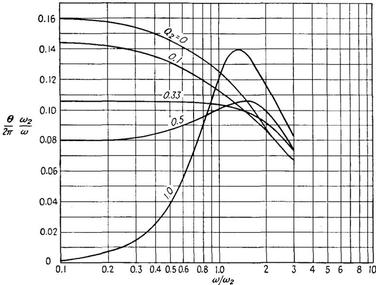
FIG. 6-6. Dimensionless curves of  $\theta/\omega$  as a function of  $\omega/\omega_2$  for shunt-compensated amplifiers.
