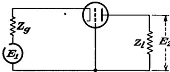
6-19. Repeat the calculations of Prob. 6-18 for the inverted amplifier of the accompanying figure.
