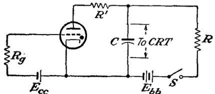
FIG. 20-6. A saw-tooth generator employing a thyatron.
