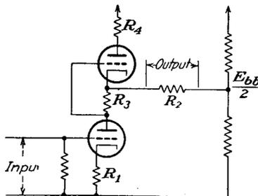
6-16. Calculate the input admittance and the output impedance of the difference amplifier when connected as shown in Fig. 6-23. Neglect tube and wiring capacitances.
