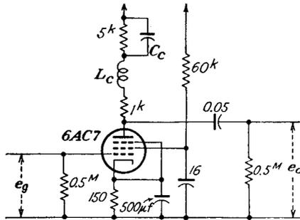
$L_c$  that will yield the same gain at the upper frequency  $f_2$  as at the mid-band. Assuming the stray wiring capacitances to be  $20 \mu\text{mf}$ , the tube capacitances of the 6AC7 are  $C_{gp} = 0.015 \mu\text{mf}$ ,  $C_{pk} = 5 \mu\text{mf}$ ,  $C_{ek} = 11 \mu\text{mf}$ . Calculate also  $f_1$  under the optimum conditions for the l-f compensation.
