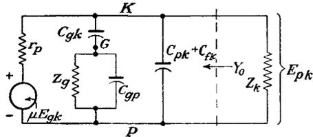
FIG. 6-14. The equivalent output circuit of the cathode follower.
