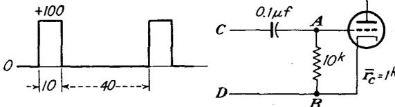
a. Estimate the reading of a d-c voltmeter which draws negligible current when connected between points C and A in the circuit in the sketch.
