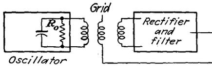
tube is removed indicates that with an input of  $E_p = 8$  volts rms the potentials are  $E_g = 0.4$  volts rms,  $E_{cc} = 11.4$  volts d-c. What is the value of  $R_o$  for the bias to adjust itself to  $-7.5$  volts?
