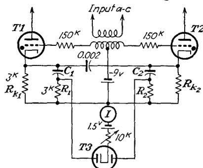
causes  $C_1$  to charge through the parallel paths  $R_1$  and one plate of the rectifier T3. The average diode current is indicated by the meter in series with the diode cathode. The diode current is proportional to the frequency, over the range for which  $C_1$  and  $C_2$  charge "fully" in less than the time of one half cycle of the impressed voltage. For the circuit shown, the calibration of the instrument is linear to approximately 7,000 cps.
