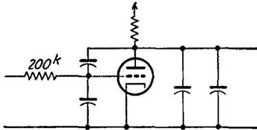
7-6. A saw-tooth voltage is applied to the circuit shown in the diagram for this problem. Calculate and sketch the output voltage during one complete period.
