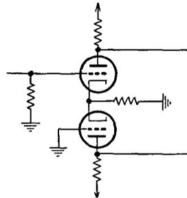
FIG. 20-27. A cathode-coupled paraphase amplifier.
