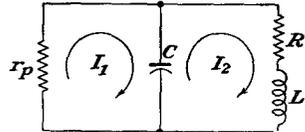
FIG. 12-26. The basic equivalent circuit of a negative-resistance oscillator.
