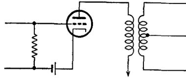
FIG. 9-24. A simple driver circuit for a push-pull amplifier.
