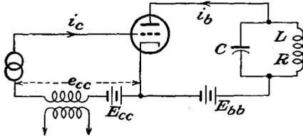
FIG. 15-12. A grid-bias modulated class C amplifier.
