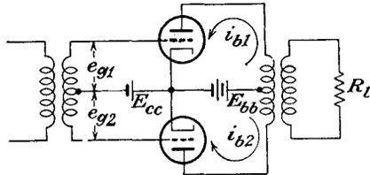
FIG. 9-14. The basic push-pull circuit.
