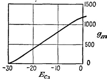
diagram for this problem. A beating oscillator signal of 24 volts peak, which causes a bias of  $-20$  volts to be developed, is applied to grid 3. The incoming signal of  $100 \mu$ v is applied to grid 1, which is maintained at a bias of  $-6$  volts. Calculate the conversion transconductance under these conditions.
