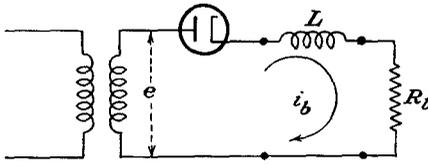
FIG. 14-1. Half-wave rectifier circuit with choke filter.
