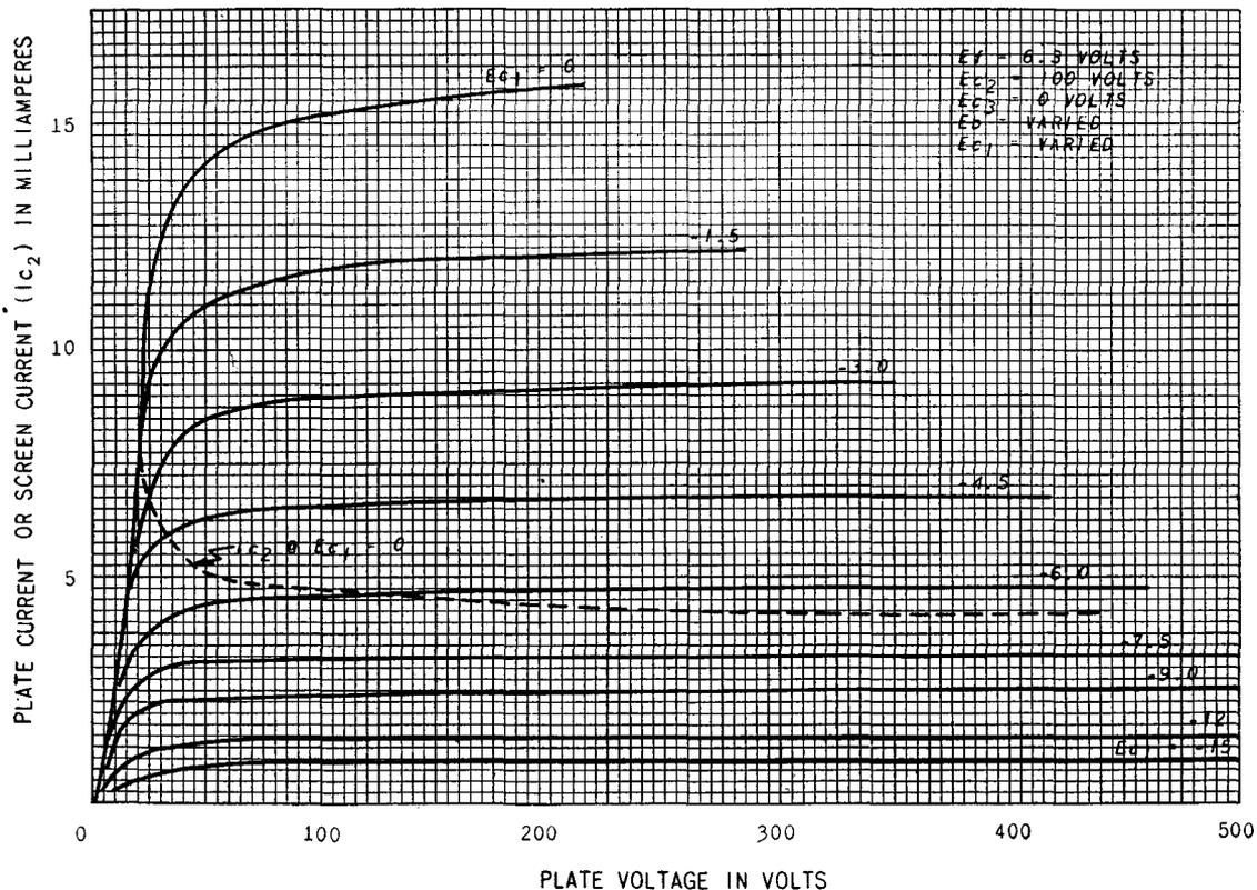
Fig. B-13. 6SK7 variable-mu pentode.
