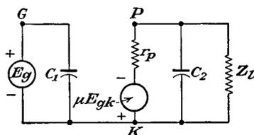
FIG. 4-7. The ideal equivalent circuit of a tetrode amplifier.
