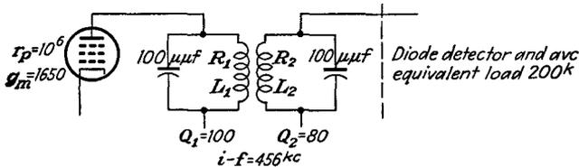
The rms potential across the secondary feeding the detector-automatic-volume-control circuits must be 10 volts.
