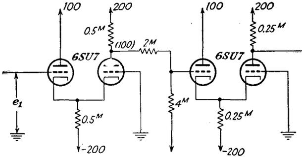
FIG. 6-24. A multistage d-c amplifier employing difference amplifiers.
