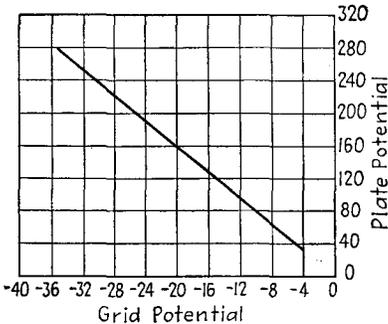
FIG. 2-27. Critical grid characteristic of an 884 argon-filled thyratron.
