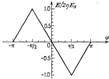
FIG. 22-17. The output of the phasemeter of Fig. 22-16.
