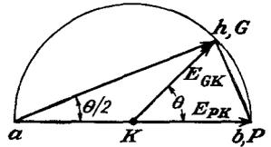
**13-8. D-C Bias Control.** The magnitude of the d-c or average rectified current of a thyatron may be controlled by applying a d-c bias to the grid of the tube and controlling its magnitude. The plate supply must be an a-c potential. The situation is best understood by reference to Fig. 13-19.
