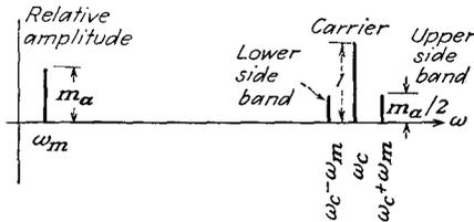
FIG. 15-2. Frequency spectrum of a sinusoidally modulated wave.
