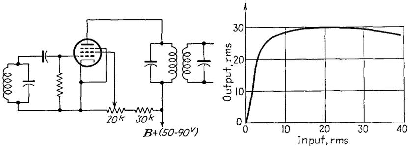
FIG. 17-28. The circuit of a limiter, and the general character of the results.
