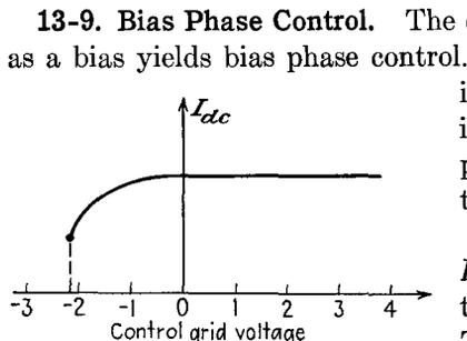
FIG. 13-20. The average plate current in a thyatron as a function of the d-c grid-bias potential.
