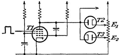
FIG. 19-26. A Miller integrator with controlled limits.
