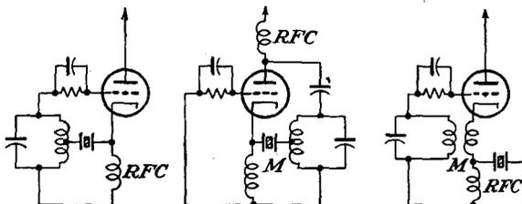
12-10. An amplitude-controlled oscillator uses a 6J5 tube. It operates at 5 megacycles. A measurement of the network and rectifier when the oscillator
