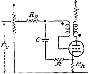
FIG. 18-20. A biased blocking oscillator.
