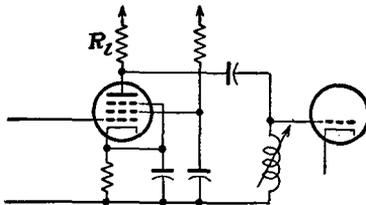
stages is 10,000, and the gain at 28.5 and 31.5 megacycles is 7,070. 6AC7 tubes are used, with  $g_m = 9,000 \mu\text{mhos}$ ,  $C_i = 11 \mu\text{mf}$ ,  $C_o = 5 \mu\text{mf}$ .
