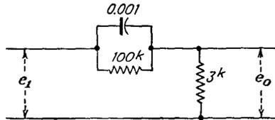
**17-12.** Calculate and plot the voltage ratio for the deemphasis circuit, shown in the accompanying figure, as a function of frequency. Plot the curve on semi-log paper.
