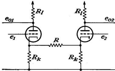
6-18. The circuit of a grounded-grid amplifier is shown. (Batteries have been omitted for convenience.) Determine the following:
