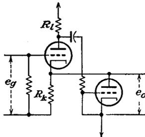
6-13. Show that the h-f cutoff of the anode-follower amplifier is approximately one-half that of the cathode follower. Show also that the l-f cutoff is approximately the same as that of the cathode-follower amplifier, for  $Z_1 = R_g$  in Circuit Fig. 6-10.
