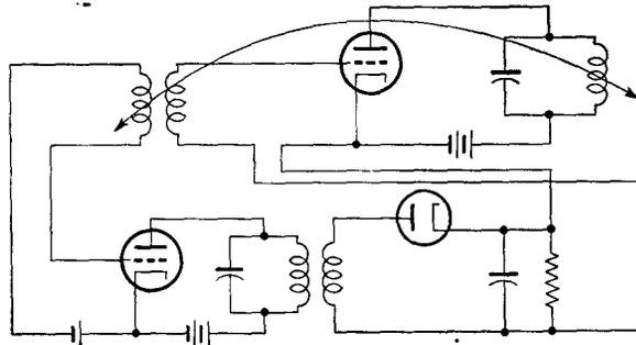
FIG. 12-15. The circuit of a linear-stabilized oscillator.
