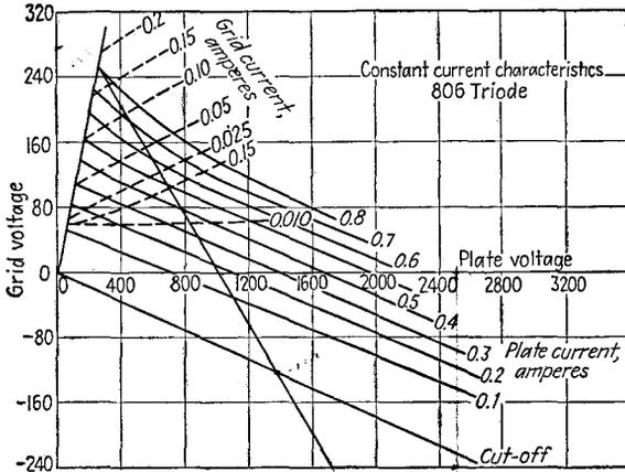
Fig. 11-12. Constant-current characteristics of an 806 triode.
