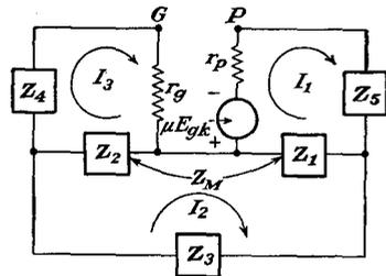
FIG. 12-9. The basic circuit of impedance stabilization.
