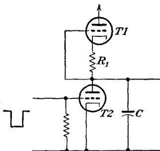
Assume that the beam resistance of  $T_2$  is  $r$ , when the tube conducts and is infinite when the gate is applied.
