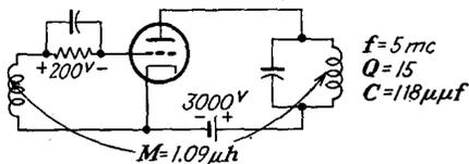
This tube is to be operated as a power oscillator in the circuit shown in the accompanying figure. Assume that  $e_{bmin} = e_{cmax}$ . Calculate the following:
