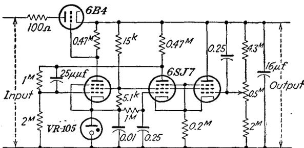
FIG. 14-23. A voltage regulator employing a difference amplifier.
