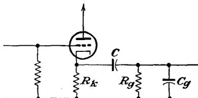
FIG. 6-10. An RC coupled cathode-follower stage.
