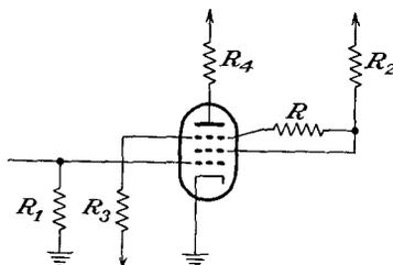
FIG. 19-19. A single pentode trigger circuit.
