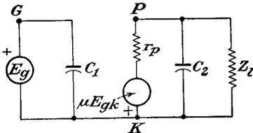
FIG. 4-8. The equivalent circuit of a pentode amplifier.
