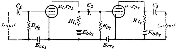
FIG. 5-1. Schematic diagram of a two-stage *RC* coupled amplifier.
