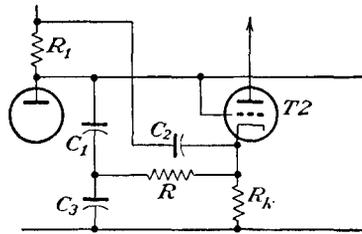
show that the voltage that appears across  $C_3$  during the saw tooth is given by
