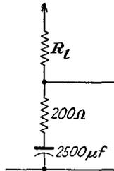
may be used as a voltage stabilizer, since, owing to the very large effective capacitance across the output, a ripple of almost any frequency that appears in  $E_{bb}$  is eliminated in the output of the circuit.
