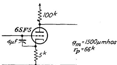
5-17. The general current feedback circuit, as viewed from the output terminals for output impedance measurements, is illustrated. Analyze this circuit, and verify Eq. (5-57).
