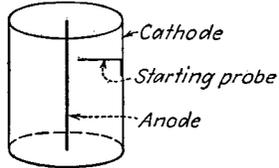
FIG. 2-20. Electrode structure in a VR tube.
