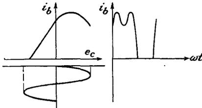
FIG. 7-12. Formation of a square wave by saturation and cutoff limiting. The overdriven amplifier.
