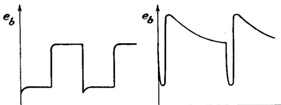
FIG. 18-1. The output-voltage wave forms in the multivibrator and in the blocking oscillator.
