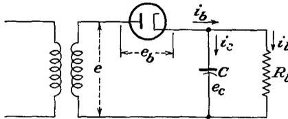
FIG. 14-4. A single-phase half-wave capacitor filtered rectifier.
