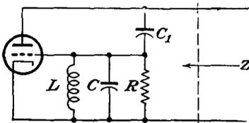
17-6. Given the reactance-tube circuit in the figure. Show that, if the reactance of  $C$  is negligible at the operating frequency and if  $\omega L \gg R$ , the effective input impedance results from an inductance  $L/g_m R$ .
