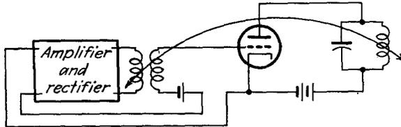
FIG. 12-14. A linear-stabilized oscillator.
