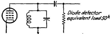
The equivalent output circuit is illustrated. The tank is tuned to  $f_0 = 1$  megacycle,  $L = 0.5$  mh,  $Q = 60$ . Assume for the 6SK7 that  $r_p = 10^6$ ,  $g_m = 2,000$   $\mu$ mhos. Determine
