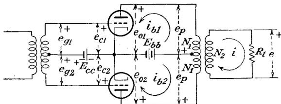
FIG. 9-17. The potentials in the push-pull amplifier.
