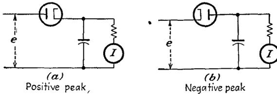
FIG. 22-5. Peak-reading voltmeters.
