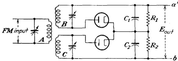
FIG. 17-30. A discriminator employing two stagger-tuned circuits.
