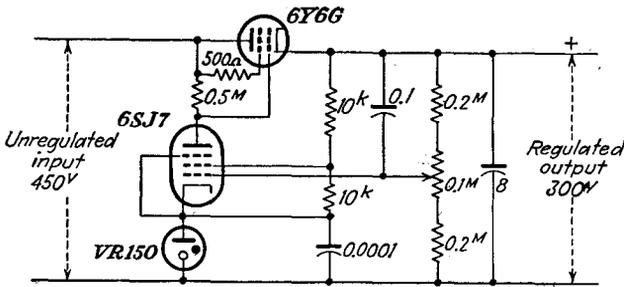
FIG. 14-21. An electronically regulated power supply.
