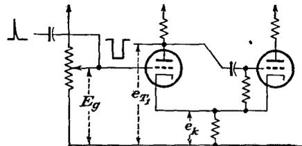
FIG. 19-6. A cathode-coupled gate with the grid of *T1* tied to a positive bias  $E_g$ .
