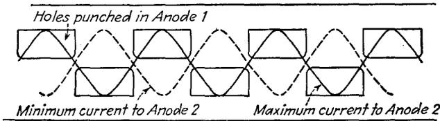
FIG. 17-25. A developed portion of anode 1.
