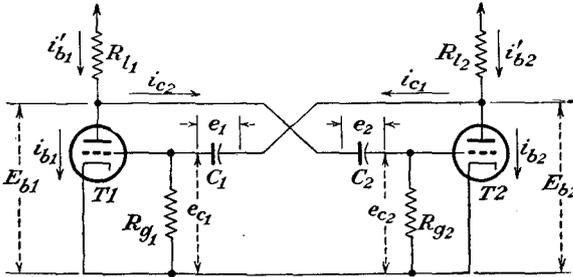
FIG. 18-3. The plate-coupled multivibrator, with voltages and currents labeled.
