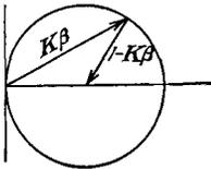
FIG. 5-24. A plot of  $|1 - K\beta| = 1$  in the complex plane.
